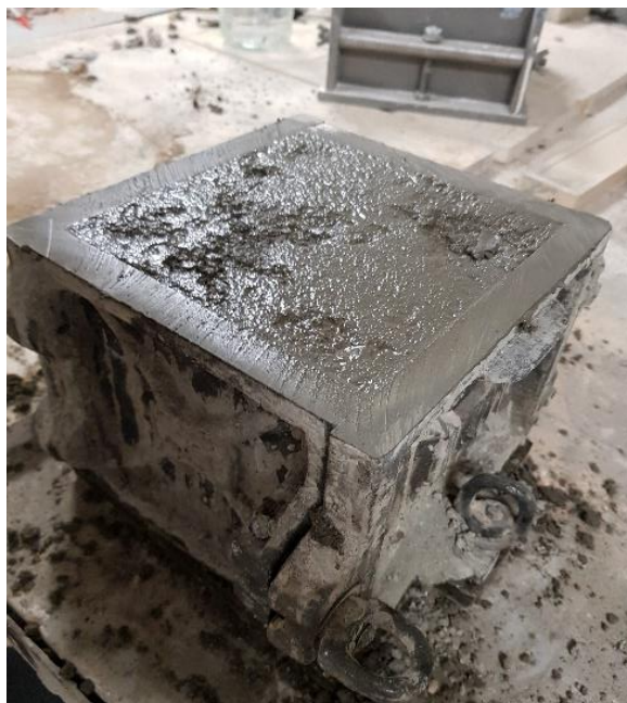
Figure 11. A 150 millimeter mold filled with concrete
